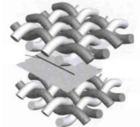
Figure2 Schematic diagram of the hot wire method
